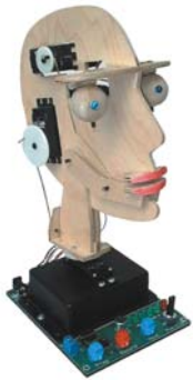
Alex animated head can be programmed using the development board and the actuators panel
