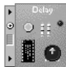
When the arrow points into a subsystem block, the Connector provides an **input** signal.
