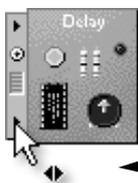
Click on a Connector arrow with the right mouse button to change the direction in which the signal flows.
