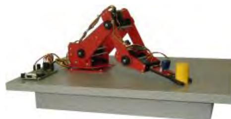
**MODULO MACCHINA CON CONTROLLO A TRE ASSI**
